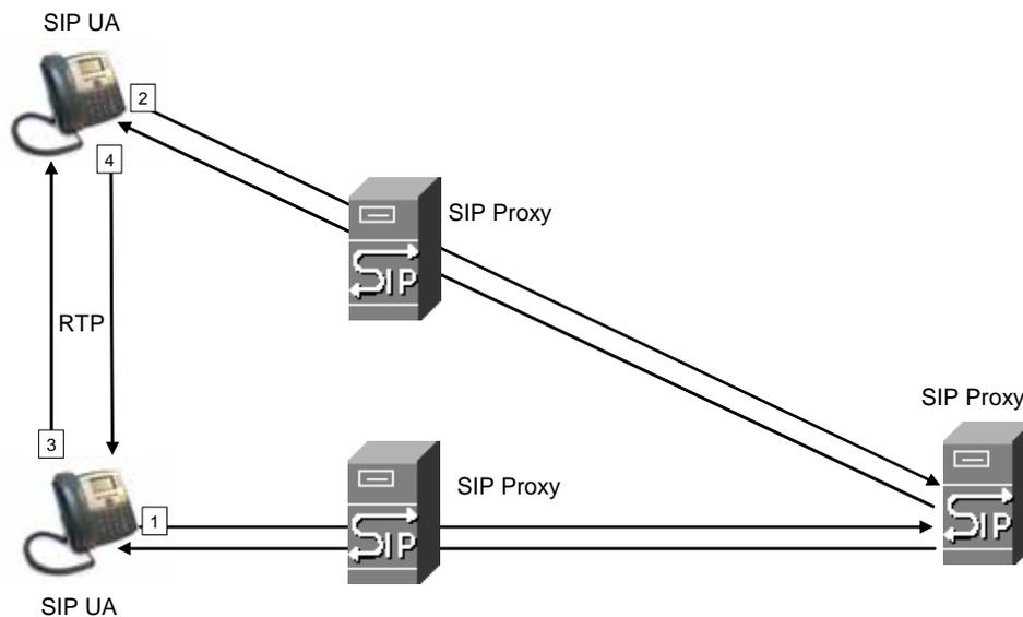
In a SIP VoIP network, when the SIP proxy receives a request from a UAS for a connection and it does not know the location of the UAC, it forwards the message to another SIP proxy in the network. Once the UAC is located and the response is routed back to the UAS, a direct peer-to-peer session is established between the two UAs. The actual voice traffic is transmitted between UAs over dynamically assigned ports using the Real-time Protocol (RTP).
