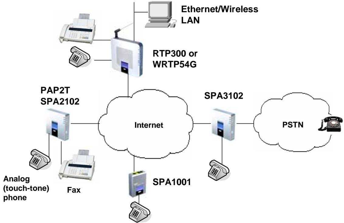
Each Linksys ATA is an intelligent low-density Voice over IP (VoIP) gateway that enables carrier-class residential and business IP Telephony services delivered over broadband or high-speed Internet connections. Linksys ATAs maintain the states of all the calls it terminates and makes the proper reaction to user input events (such as on/off hook or hook flash). Because the ATAs use the SIP standard, there is little or no involvement by a “middle-man” server or media gateway controller.
