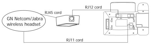
The Wireless Headset Adapter is the connection between the T28/T26 IP phone and the Plantronics wireless headset.
