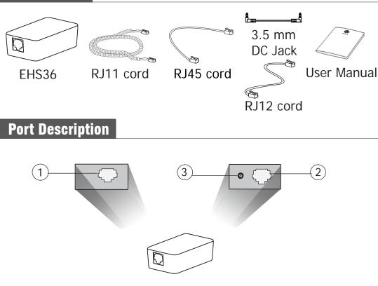
Port ①: Connect with the IP Phone EXT port or Expansion Module port (expansion module connected to the phone) through RJ12 cord.
