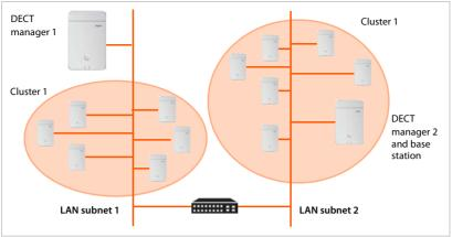
In installations with multiple DECT managers, handover and roaming between base stations of different DECT managers are possible when the clusters are synchronised. Load balancing is not possible. For more information on this, refer to Section **Using multiple DECT managers**  $\rightarrow$  P. 16.
