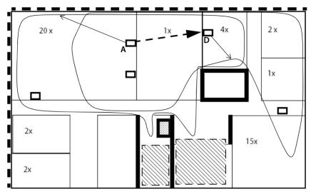
In the example, limitation lines are drawn for the wireless coverage for base stations A and D. The overlap areas are very good for both stations; synchronisation is also guaranteed between A and D. However, the measurement results of the other stations must be used to check whether a further base station is required in the shaded areas.
