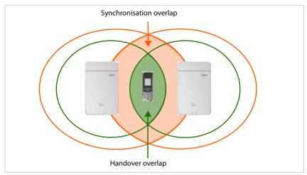
A sufficiently high number of overlapping zones between neighbouring cells must be ensured.
