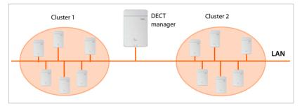
For installations in different LAN subnets, multiple DECT managers with one DECT manager per subnet are required. The DECT manager function can be installed in parallel on the same device (depending on the capacity of the local base station). Multiple DECT managers are also required when the requirement is to connect more than 250 handsets or provide more than 60 connection channels.
