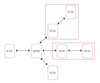
As shown above, the total number of the four repeaters in cascade setup and two repeaters in star setup is six.
