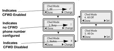
In the above example, CFWD All is enabled as indicated by a check mark ( $\checkmark$ ), CFWD Busy is enabled but no call forward phone number configured as indicated by a !, and CFWD NoAns is disabled, as indicated by an **X**.
