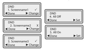
In the above example, Screenname1 and 3 have DND ON as indicated by a check mark ( $\checkmark$ ). Screenname2 has DND off as indicated by an **X**. Items 4 and 5 allow you to disable or enable DND on all accounts, respectively.
