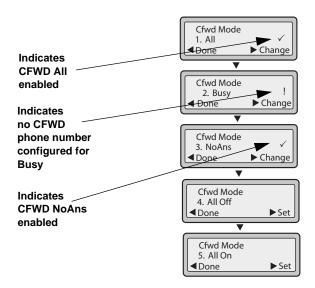
In the above example, the account has **CFWD All** and **CFWD NoAns** enabled as indicated by a check mark ( $\checkmark$ ). The **CFWD Busy** setting is enabled for the account but has no call forward phone number configured as indicated by a **!**.
