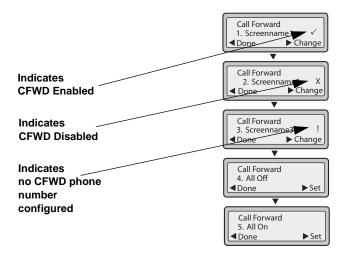
In the above example, Screenname1 has one or more CFWD states enabled as indicated by a check mark ( $\checkmark$ ). Screenname2 has one or more CFWD states disabled as indicated by an **X**. Screenname3 has one or more CFWD states configured but a specific state has no call forward phone number configured as indicated by a **!**. Items 4 and 5 allow you to disable or enable CFWD on all accounts, respectively.
