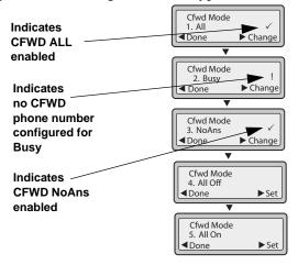
In the above example, the account has CFWD All and CFWD NoAns enabled as indicated by a check mark ( $\checkmark$ ). The CFWD Busy setting is enabled but no call forward phone number is configured as indicated by a !.
