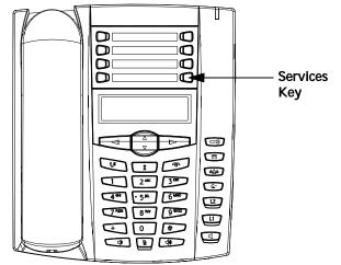
The 6730i allows you to configure a Services key that, when pressed on the phone, displays the Services menu. The Services Menu can also be accessed via the IP Phone UI at the location, *Options->Services*. The Services key can access any XML applications setup by your System Administrator. Contract your System Administrator for more information.
