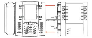
The M675i provides 10 softkeys in each column (totaling 20 keys) on the keypad. The M675i also provides 3 keys at the bottom left of the unit. These keys represent
