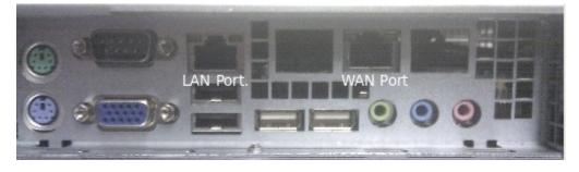
The SARK1200 has two (2) RJ45 Ethernet ports assigned as follows (when viewed, left to right, from the rear of the enclosure);
