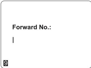
There will be a number 9 on the bottom left corner of the screen, indicating the current input mode. Press **#** button to cycle through 9 (numbers), **A** (upper case letters), and **a** (lower case letters) for your desired input mode.
