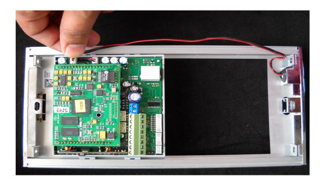
3. Fix the push button module on the frame and connect the 2 pin connector from LT on sip module to INPUT on push button as seen below.
