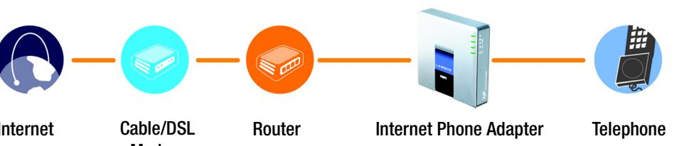
**A** Connect the included Ethernet network cable to the ETHERNET port of the Internet Phone Adapter.
