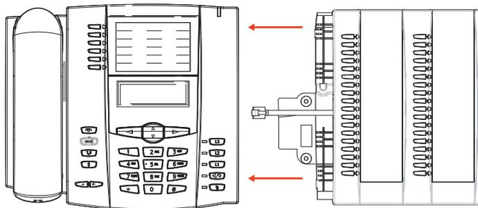
The M670i provides 18 keys in each column (totaling 36 keys) on the keypad. Each key provides an LED for indicating call status. The M670i provides a paper label for convenient key labeling.
