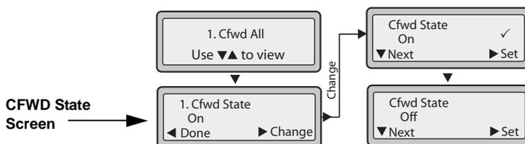
5. Press the **CHANGE** key in the CFWD State screen. Press **NEXT** to toggle the state of the CFWD state ON or OFF. In the example in Step 4, you press **NEXT** to change the option to **OFF**.
