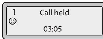
For on-hold calls, the timer displays as running and the Line and main LEDs flash.
