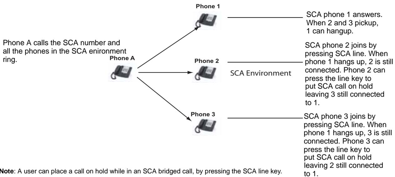
Using the example above, when a call comes into Phone 1, Phone 2 and Phone 3 can pickup the same call by pressing the SCA line key. Phone 2 and 3 display the call they are bridging into on the LCD of the phones. Existing SCA parties in a bridge or one-to-one call hear an audible beep when another party has joined the call.
