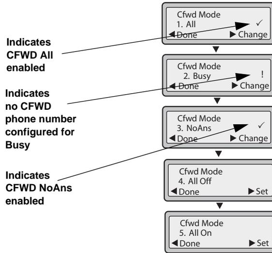
In the above example, the account has **CFWD All** and **CFWD NoAns** enabled as indicated by a check mark (✓). The **CFWD Busy** setting is enabled for the account but has no call forward phone number configured as indicated by a !.
