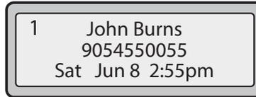
The **Idle State** screen lists your name (SIP screen name), extension (or phone number), and day, date, and time. The "1" in the upper corner in the above example indicates the idle screen for the first line appearance. You can use the left and right arrow keys to scroll through the idle screens for all three line appearances. The 6753i allows for scrolling up to 3 lines.
