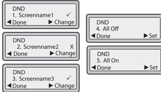
In the above example, Screenname1 and 3 have DND ON as indicated by a check mark (✓). Screenname2 has DND off as indicated by an X. Items 4 and 5 allow you to disable or enable DND on all accounts, respectively.
