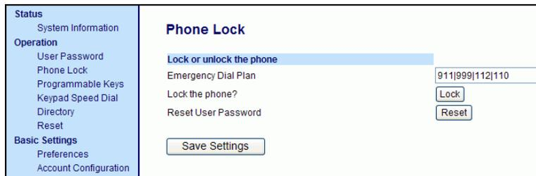
2. In the "**Emergency Dial Plan**" field, enter the 3-digit number used in your local area to contact emergency services. For multiple numbers, enter a "|" between each emergency number. For example:
