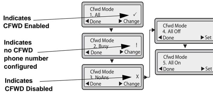
In the above example, CFWD All is enabled as indicated by a check mark (✓), CFWD Busy is enabled but no call forward phone number configured as indicated by a !, and CFWD NoAns is disabled, as indicated by an X.
