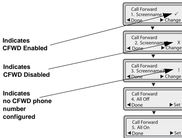
In the above example, Screenname1 has one or more CFWD states enabled as indicated by a check mark (✓). Screenname2 has one or more CFWD states disabled as indicated by an **X**. Screenname3 has one or more CFWD states configured but a specific state has no call forward phone number configured as indicated by a **!**. Items 4 and 5 allow you to disable or enable CFWD on all accounts, respectively.
