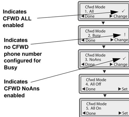
In the above example, the account has CFWD All and CFWD NoAns enabled as indicated by a check mark (✓). The CFWD Busy setting is enabled but no call forward phone number is configured as indicated by a !.
