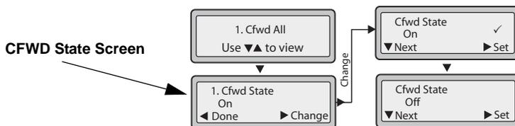
5. Press the **CHANGE** key in the CFWD State screen. Press **NEXT** to toggle the state of the CFWD mode ON or OFF. In the example in Step 4, you press **NEXT** to change the option to OFF.
