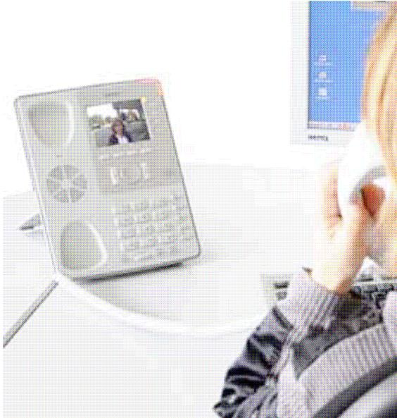
With the desktop telephone snom 820, the video image of the CP- CAM is directly shown on the phone display.
