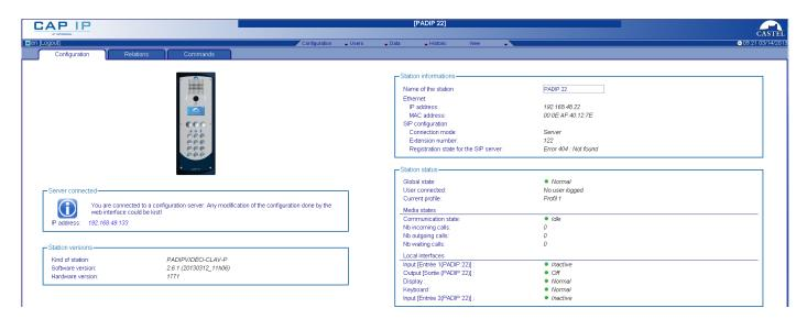
Web server provides information on the station and configure. To have all the functions, go on to display/full display. Online help is accessible from any menu gives information on the various functions of the web server.
