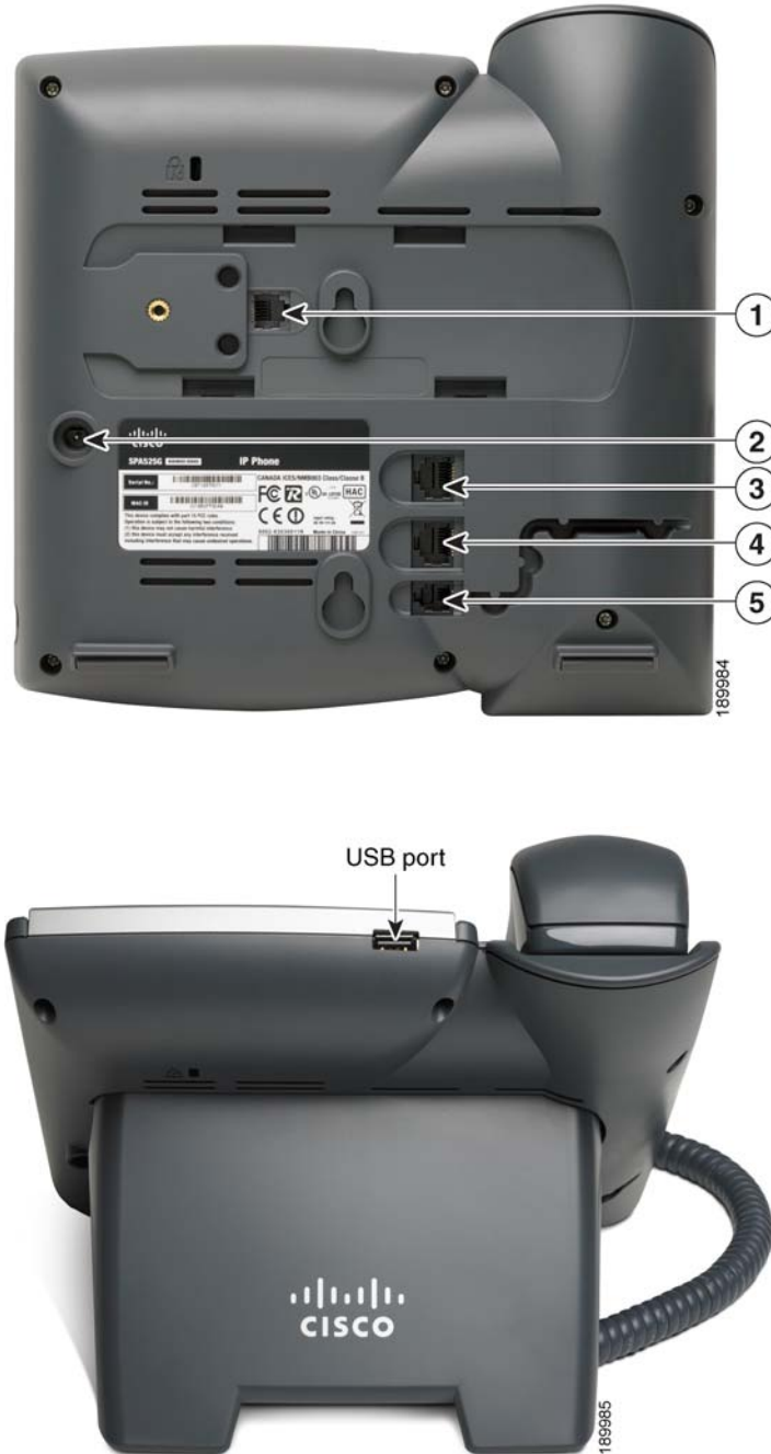
Figure 1 Cisco SPA525G IP Phone Connections
