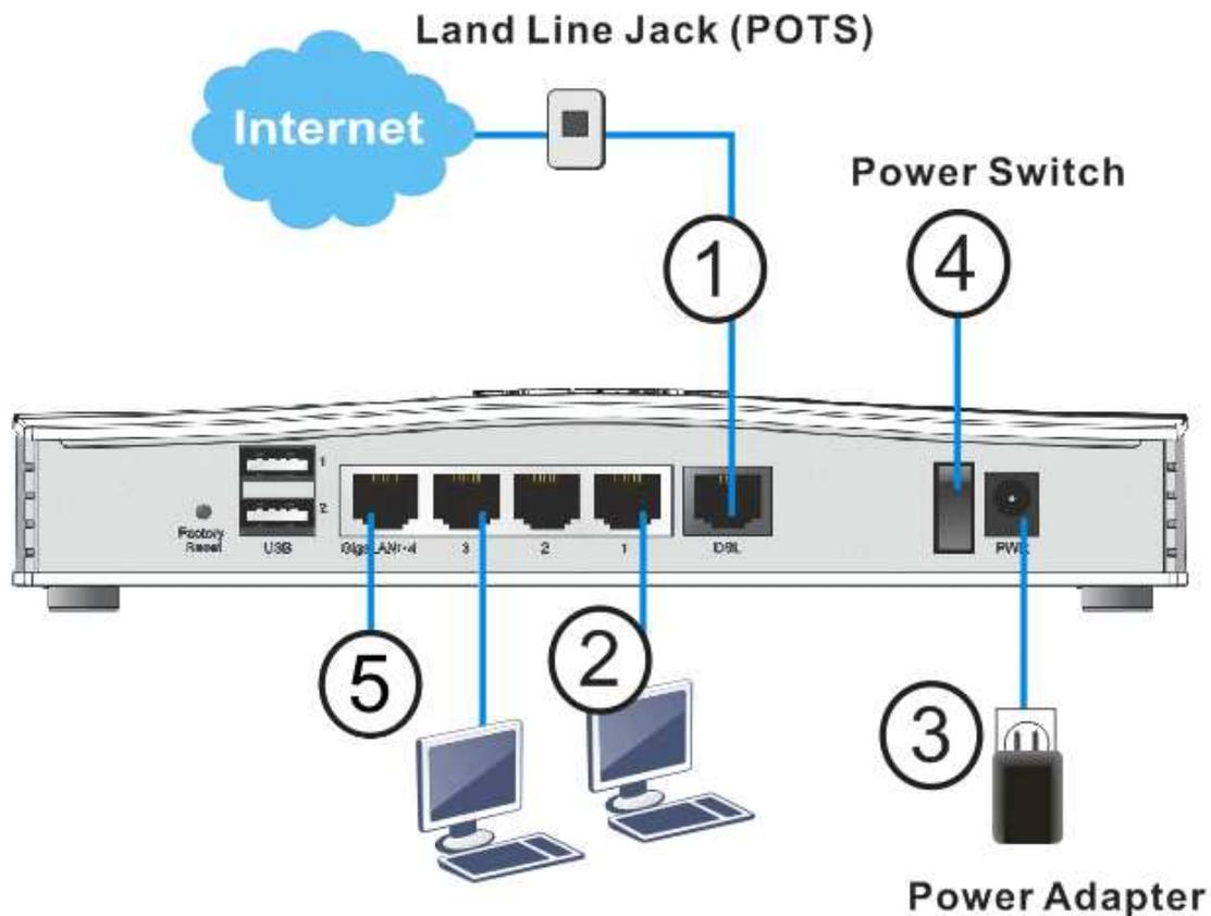
1. **ADSL/VDSL Connections:** Connect the DSL port to the Modem or DSL port of the external splitter/microfilter (not supplied) with the RJ-11 line cable. In some cases, your RJ-11 DSL socket will be built-into your phone line socket on the wall and you won't have a separate microfilter/splitter.
