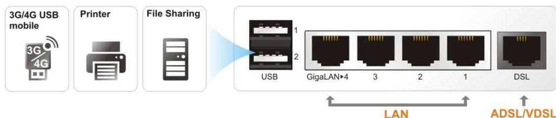
A 4-port Gigabit Ethernet switch on the LAN side provides high speed connectivity for your computers or network storage (NAS) devices and can connect a VigorAP wireless access point or network switch with 802.1Q VLAN tagging. Comprehensive security features include content filtering, web application controls and an object based firewall management system.
