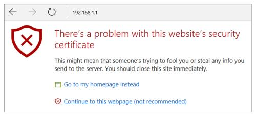
Most other browsers will present equivalent warnings. In each case, following the prompts/links will allow you to access the router's web interface. It is still encrypted with SSL/TLS.
