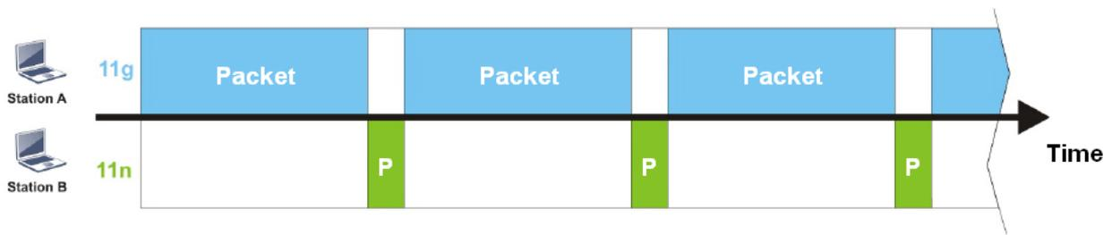
To improve this problem, Airtime Fairness is added for VigorAP 802. Airtime Fairness function tries to assign *similar airtime* to each station (A/B) by controlling TX traffic. In the following figure, Station B(11n) has higher probability to send data packets than Station A(11g). By this way, Station B(fast rate) gets fair airtime and it's speed is not limited by Station A(slow rate).
