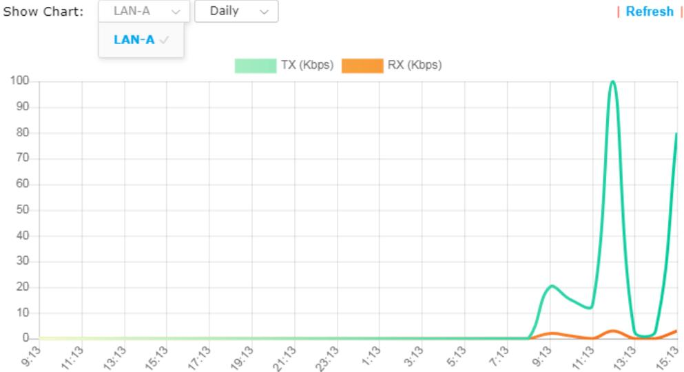
The horizontal axis represents time; the vertical axis represents the transmission rate (in kbps).
