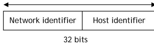
With the classful addressing, it divides IP address into three classes, class A, class B and class C. The rest of IP addresses are for multicast and broadcast. The bit length of the network prefix is the same as that of the subnet mask and is denoted as IP address/X, for example, 192.168.1.0/24. Each class has its address range described below.
