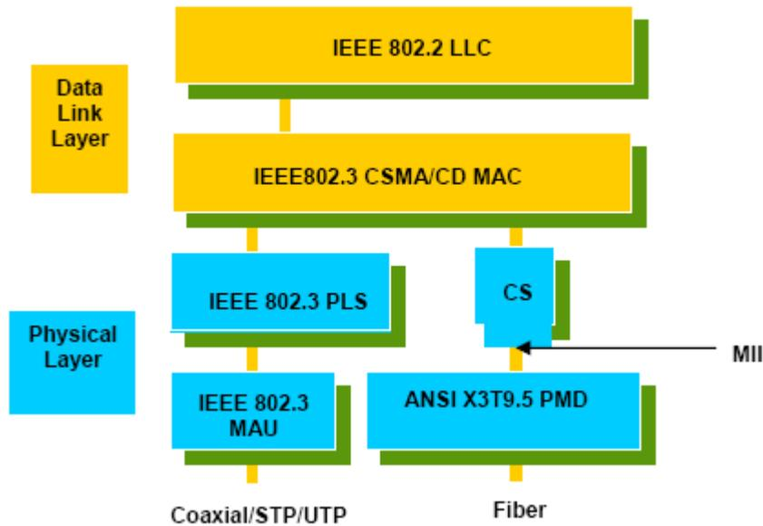
This above diagram shows the Ethernet architecture, LLC sub-layer and MAC sub-layer, which are responded to the Data Link layer, and transceivers, which are responded to the Physical layer in OSI model. In this section, we are mainly describing the MAC sub-layer.
