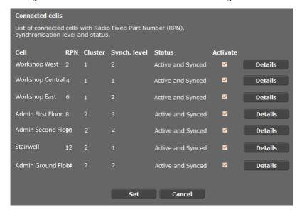
The **Base station settings** page shows a table of all connected base stations with the name, RPN (Radio Part Number, number of the cell on the DECT network), cluster number, synchronisation level and status.
