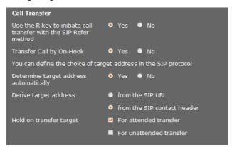
Participants can transfer a call to another participant as long as the PABX/provider supports this function. The call is transferred using the handset menu (via the display key) or using the R key ( > page 37).
