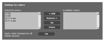
Both parties involved in a phone connection (caller/sender and recipient) must use the same voice codec. The voice codec is negotiated between the sender and the recipient when establishing a connection. You can select the voice codecs to be used for this VoIP account and specify the order in which the codecs are to be suggested when a VoIP connection is established.
