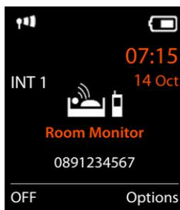
The destination number is displayed in idle display when the room monitor is activated.
