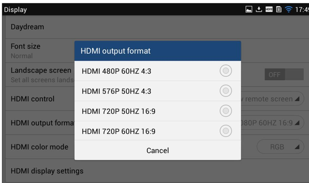
Figure 155: Settings->Display->HDMI Output Format
