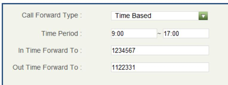
The screenshot shows a web form for configuring time-based call forwarding. It includes four fields: 'Call Forward Type' (dropdown set to 'Time Based'), 'Time Period' (input fields for '9:00' and '17:00' with a tilde separator), 'In Time Forward To' (input field with '1234567'), and 'Out Time Forward To' (input field with '1122331').
