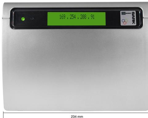
The appliance can be wall or bench mounted. The dimensions are 34mmx172mmx234mm(HxLxW).
