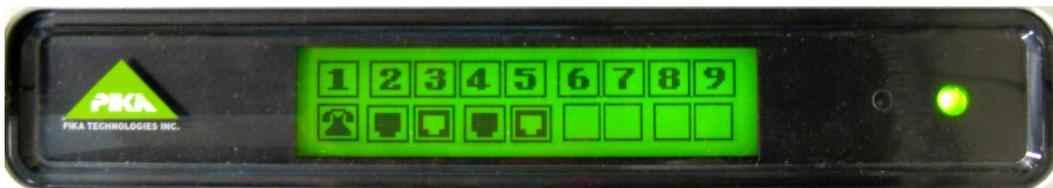
The following example shows the display where channel one (FXS), three (FXS) and eight (FXO) have calls in progress. Channel nine (FXO) is active but is currently idle. Channels six and seven (FXO) are not connected.
