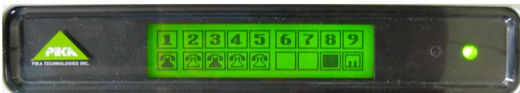
The following example shows the display where channel one (FXS) is idle, channel two (GSM) has a call in progress, and channel three (GSM) is disconnected (no SIM card plugged in).
