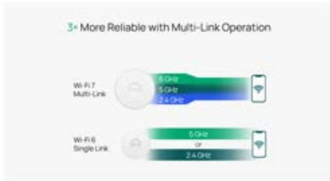
Wi-Fi 6 devices primarily rely on a single link for data transmission. In contrast, Wi-Fi 7 introduces Multi-Link Operation (MLO), enabling devices to utilize multiple links simultaneously, thereby achieving higher throughput, lower latency, and improved reliability.
