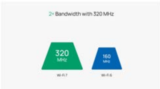
With 320 MHz ultra-wide channels, Wi-Fi 7 doubles the bandwidth of Wi-Fi 6's 160 MHz and the number of subcarriers, delivering dramatically higher data transfer rates.
