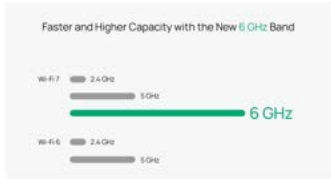
The new 6 GHz band offers a larger spectrum and cleaner channels compared to traditional bands, delivering higher capacity, faster connectivity, and less interference.
