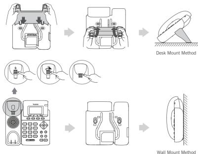
Note: The hookswitch tab has a lip which allows the handset to stay on-hook when the IP phone is mounted vertically.
